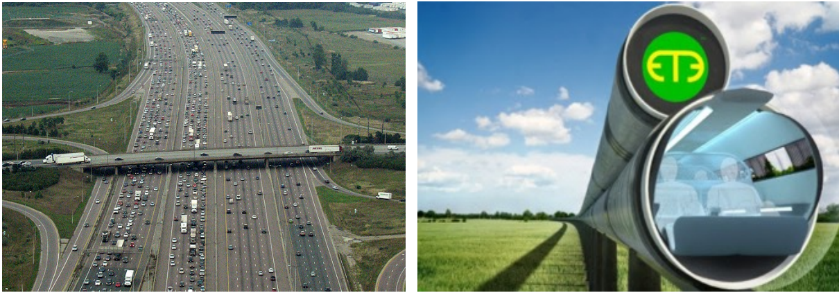
Figure 3: Examples of the two-way transport connection (with the same capacity, 1 million passengers/day) comprised of: conventional 18-lane freeway for 100 km/h that is 72 m-wide (left, [https://commons.wikimedia.org/wiki/File:Highway_401.png]) and operated at load factor of 0.5; a pair of ET3 vacuum tubes for 600 km/h operated at load factor of 0.16 (right, the elevated by 6 m tubes have diameter of 1.5 m each and the overall footprint of 1x1 m 2 every 25 m). Such ET3 connection costs less than 1/4 of the freeway connection and fits in one lane. Notably, the same ET3 connection operated at full load is close in capacity to a 100-lane freeway, such as the 400-m wide Beijing-Hong Kong-Macau Expressway (not shown).
